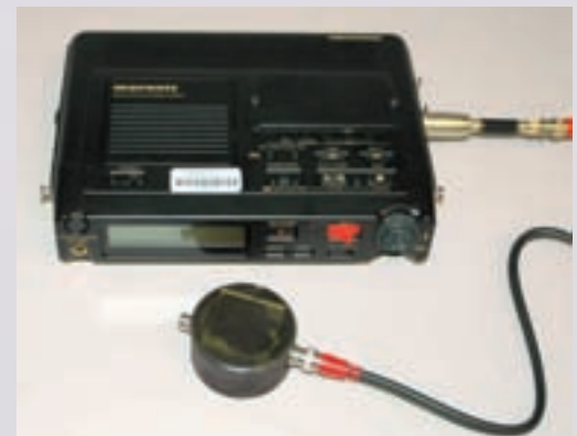
An early prototype of Moore's photosensor connected to a solid state digital recorder. This set up is used for field recordings of flying insects.
