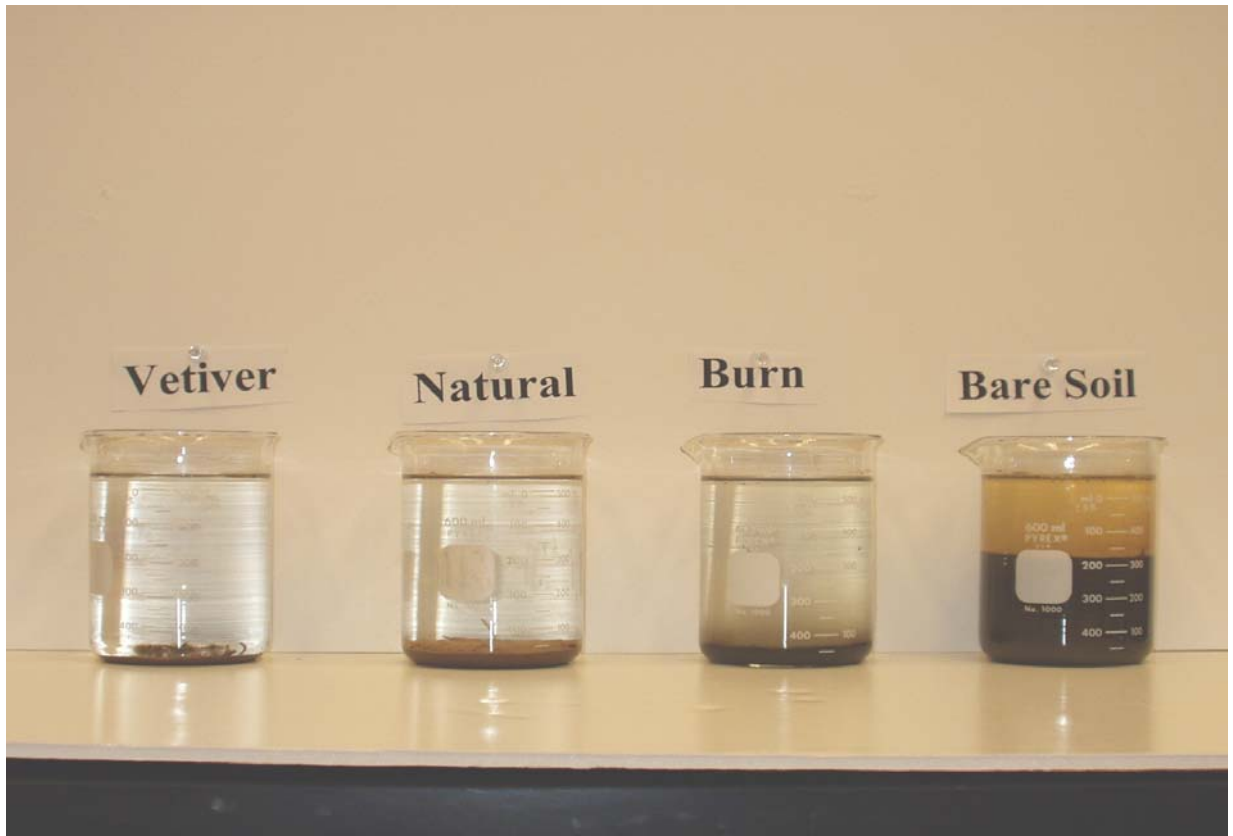
Fig. 4: Runoff samples illustrating the differences in water quality leaving the different experimental plots after a major storm event.
